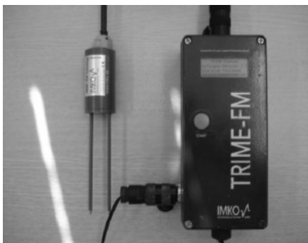
Fig. 6. TDR (Time Domain Reflectometry) sensor for unfrozen water content measurement
