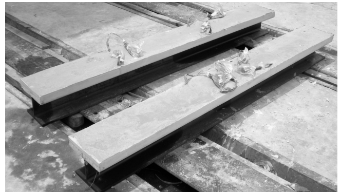
Fig. 4 Manufactured UHPC composite girder
