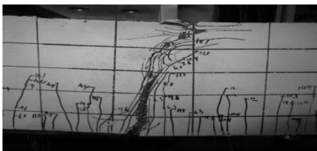
Fig. 7 Flexural failure of beam B-R4
