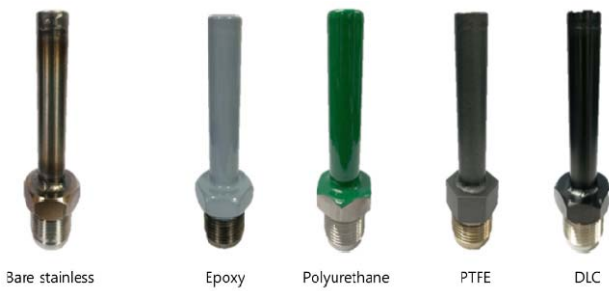
Figure 6: Various cold fingers through processed coating.
