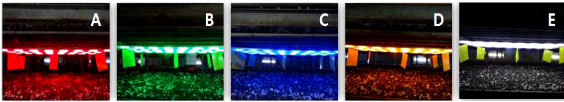
Fig. 1. lights emitting diode(LED) lights and yellow sticky traps were used for attractions of Lycoriella ingenua in Agaricus bisporus . A; Red light(627 nm), B; Green light(528 nm), C; blue light(464 nm), D; Yellow light(590 nm), E; White light(No fixed wavelength)
