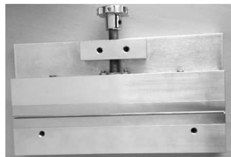
Fig. 2 Welding jig manufactured for Ti tube
