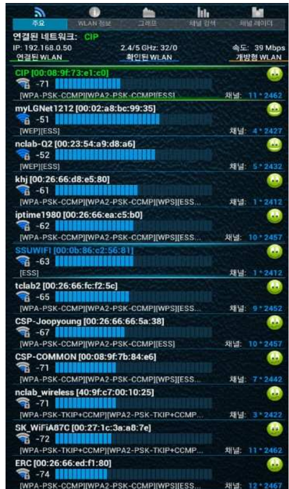
Fig. 2 Actual measurement of real Wi-Fi signals in a typical multi-floor building (12th floor, Hyungnam Engineering Building, Soongsil University)
