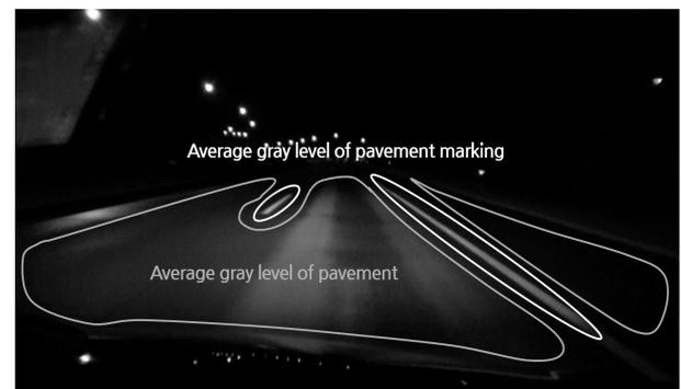
Fig. 9. Collecting Gray Level from Surface and Pavement Markings
