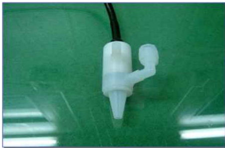
Fig. 9. Fabricated transmitter for spot spray type megasonic.
