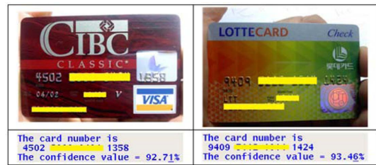
Fig. 8. Recognition results of credit cards: some numbers are deleted for reasons of security.
