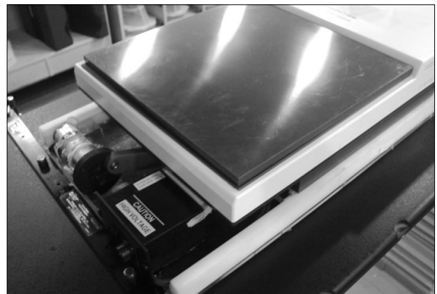
Fig. 1. To simulate the patients' respiratory motion, the moving platform was fabricated in laboratory. The solid water phantom with thickness of 1.3 cm and the MatriXX were placed on the simulating platform as shown figure. The SSD was 100 cm and the depth of measurement layer became 1.6 cm, which D max for 6 MV photon beams. We let the platform move with range of 0, 1, 2, and 3 cm and with cycle of 3.6 s.
