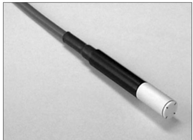
Fig. 1. Photo of the PTW 60019 microDiamond detector.
