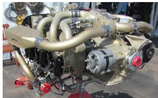
Fig. 4 Continental IO-520C Piston Engine
