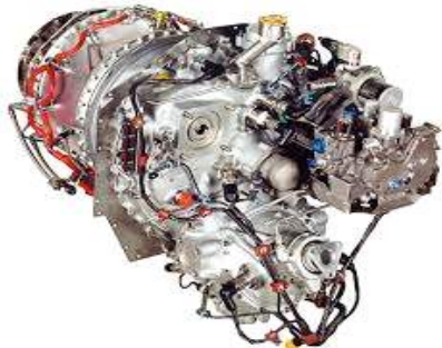
Fig. 3 PW 206C Turboshaft Engine
