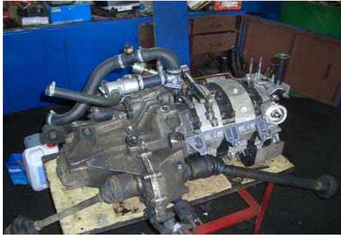
Fig. 6 VAZ 415 Rotary Engine
