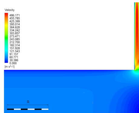
Fig. 8 Velocity contour near the nozzle exit of the drill shaped at pressure ratio of 6.92
