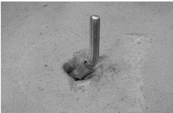
Fig. 4. Failure Mode for Embedment Depth
