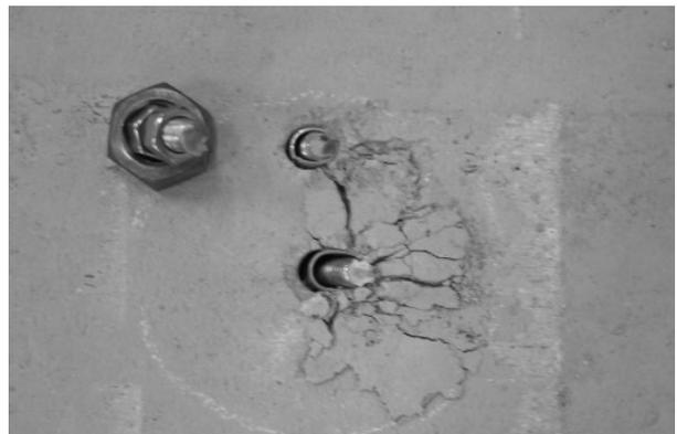
Fig. 8. Failure Mode for Anchor Interval
