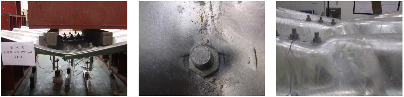
Fig. 5 Typical failure pattern under static loading
