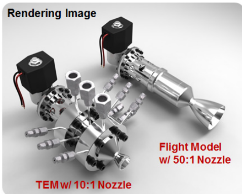
Fig. 1 Configuration of 70 N-class liquid-monopropellant hydrazine thruster.
