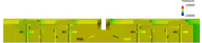
Fig. 12 Surface pressure contour (case02: semi-bogie fairing)
