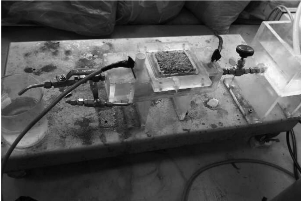
Fig. 5. A decontamination test of small electrokinetic equipment using Ca-removed water.
