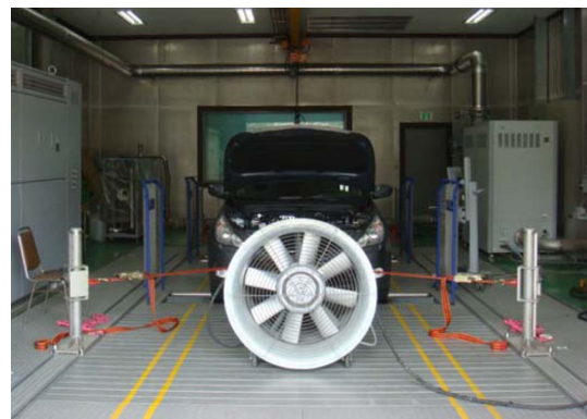
Fig. 1 Test vehicle equipped with CNG/LPLI Bi-Fuel engine
