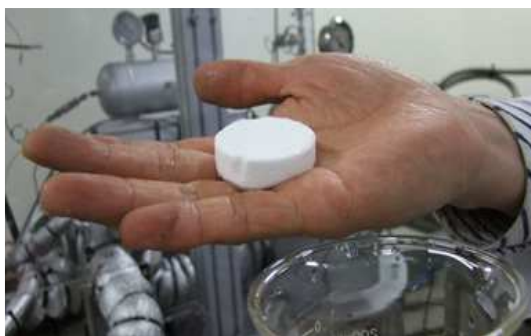
Fig. 6 Hydrate pellet from seawater
