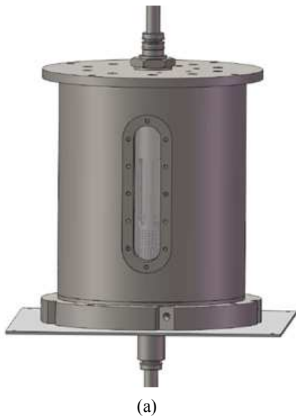
Fig. 1 Experimental apparatus for Desalination
