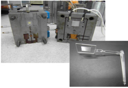
Fig. 7 Mold and the electric circuit for rapid heating of the stamper
