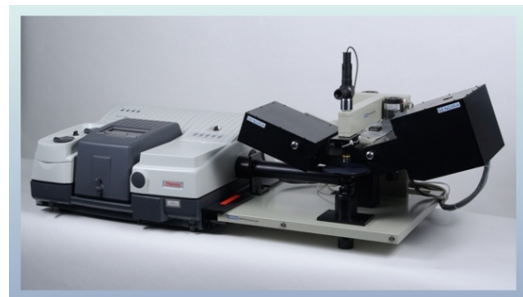
Fig. 4 FTIR analysis equipment for transmittance and refractive measurements
