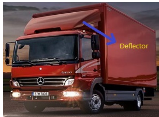
Photo 1 Deflector installed at front and upper part of truck
