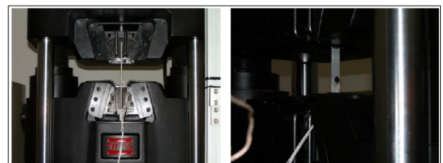
(a) Tensile test of the glass fiber (0 degree)
