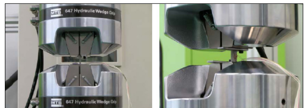
(b) Tensile test of the glass fiber (90 degree)
