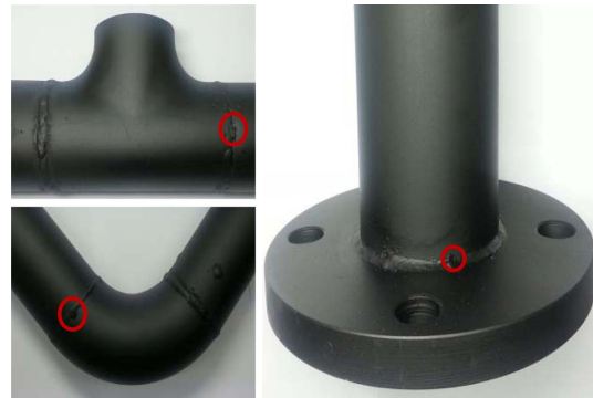
Fig. 1. Specimens for ultrasound thermography imaging.
