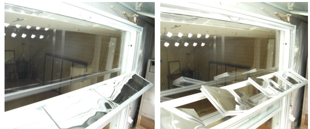
Fig. 8 Operation of light shelf module.
