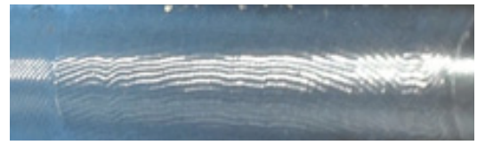
(a) With chatter vibration (depth of cut 1.2 mm, spindle speed 6,000 RPM)
