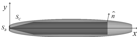
Fig. 1. Geometric definition of cavitator and supercavity
