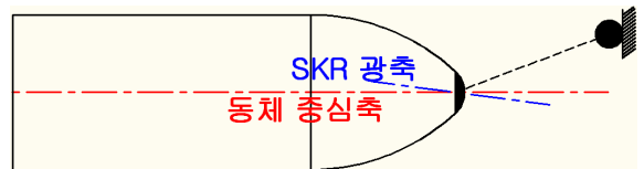
Fig. 1. Measuring Misalignment between SKR and Frame
