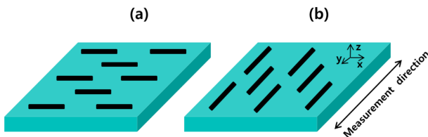
Fig. 9. CTE measurement scheme of along (a) 0° and (b) 90° to resin flow direction
