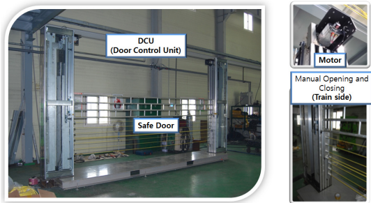
Figure 8. RPSD mock-up for test operation on the manual opening and closing algorithm
