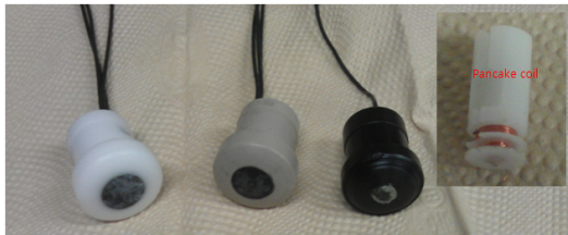
Fig. 3 Prototype ET probes for pressure tube
