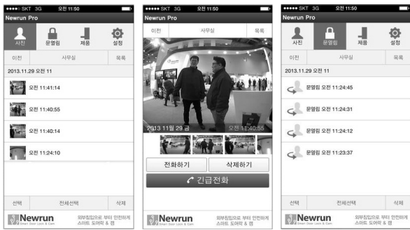
(a) (b) (c) Fig. 9. Example of Received Image and Door-Opening (a) Timeline of Received Images (b) The Selected One of Image Timeline (c) Timeline of Received Door-Opening
