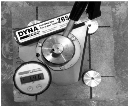
Fig. 3. Setup of bond strength test
