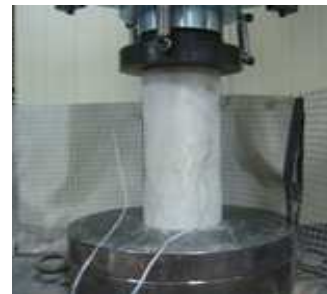
Fig. 5. Compressive strength test of PAFRC
