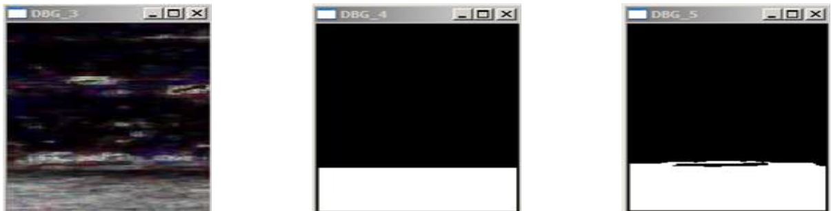
(a) Image difference (b) Boundary surface by relative Floodfill (c) Boundary surface by absolute Floodfill Fig. 4. Rippling pattern analysis by image difference and boundary surface between water and non-water areas by Floodfill algorithm
