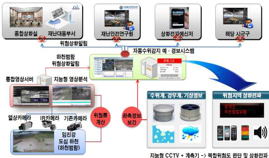
Fig. 7. Water level detection system configuration and operating scenarios by intelligent CCTV
