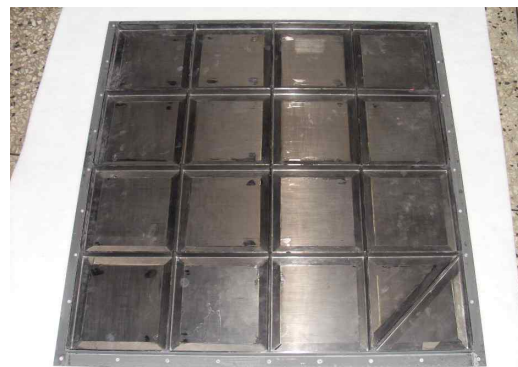
Fig. 8. Fabricated grid-stiffened structure
