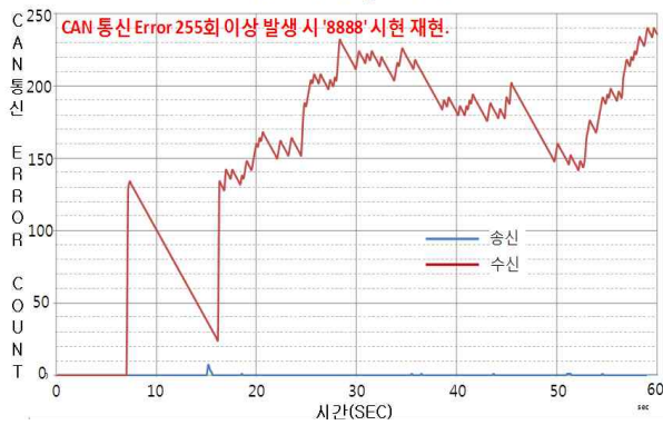
Fig. 9. CAN Communication Error Test Result in Fuel System Rig
