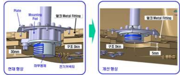
Fig. 6. Probe's Design Change in Development Phase
