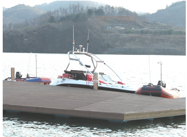
Fig.5 Traffic ships test-bed for collision avoidance : jetboat, "KOMBO"(center) and two rubber boats(left & right)
