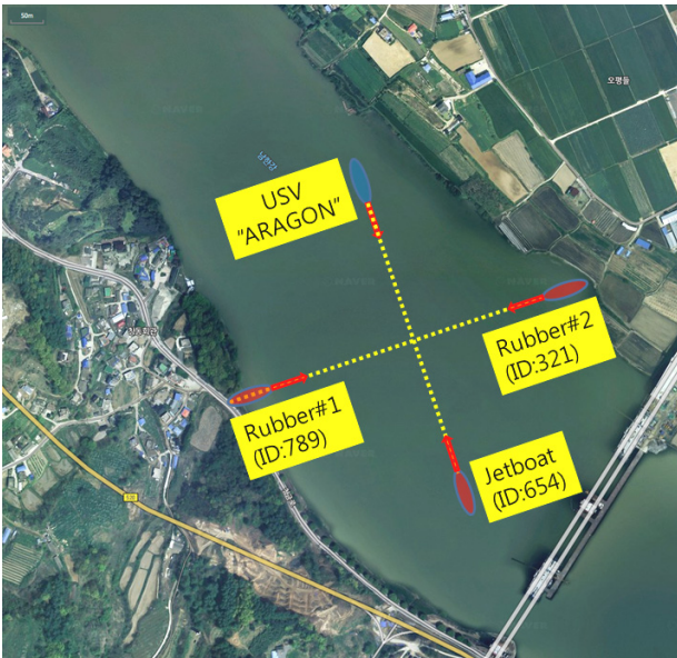
Fig.6 Scenario for test of collision avoidance
