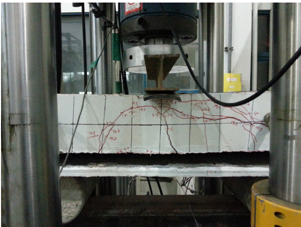
Photo 2 SMCM spalled off during the experiment
