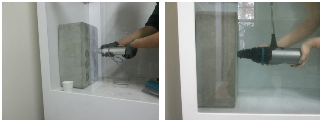
(a) Rebound Hardness Test in air condition (b) Rebound Hardness Test in under water condition
