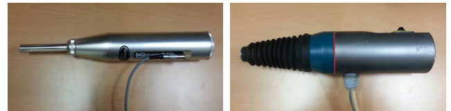
(a) Schmidt hammer before waterproof (b) Schmidt hammer after waterproof
