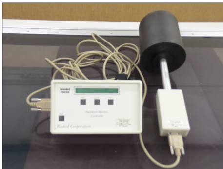
[Fig. 2] Ionization Chamber and Electrometer
