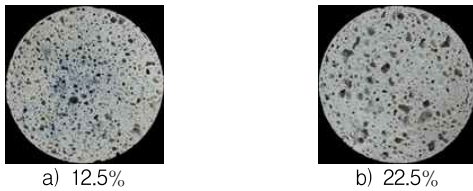
Figure 5. Cross-sectional shape of matrix according to addition ratios of NaOH
