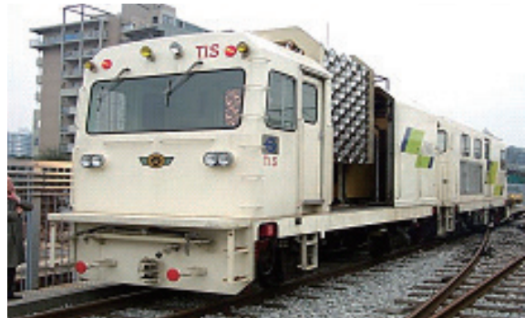
(a) Tunnel Inspection System, Japan
