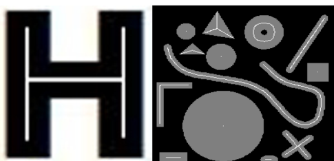
Fig. 2. The skeleton is the thinnest representation of the original pattern that preserves the topology.
