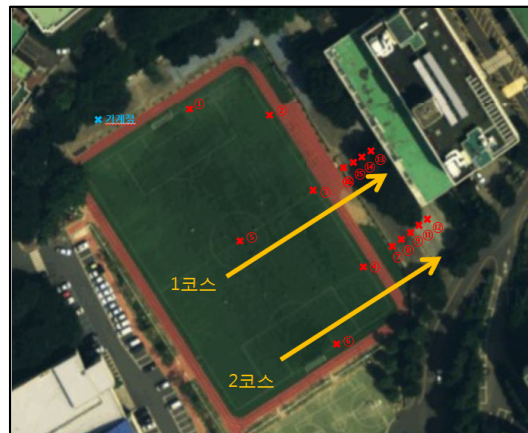
Figure 4. Check points position and surveying courses
