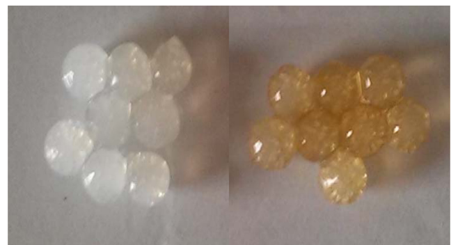
Fig. 1. Photographs of prepared chitosan beads (a) before and (b) after cellulase immobilization (average diameter = ca. 3 mm).
