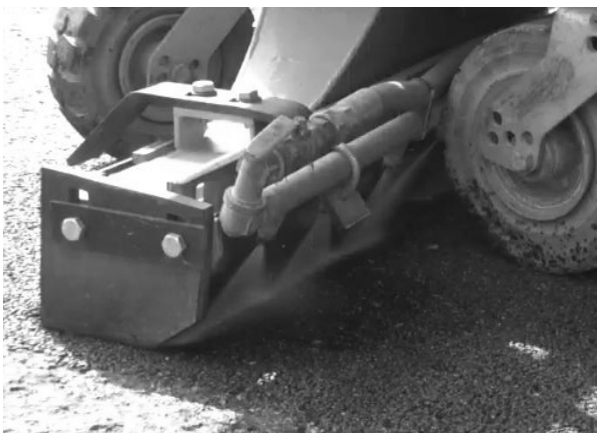
Fig. 4. Watering and Vacuum Clean Vehicle
