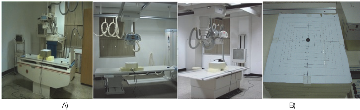
Fig. 2. A) Scattered ray containing ratio experiment of rectification type B) To use Pb disc, 'Is' fluorescence intensity measurement
